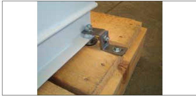
Figure 7.2. - How to pack the machine for transportation
